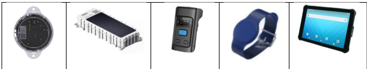
Figure 3. Sensor, geolocation device with solar panel, RFID-NFC reader, NFC watch and processing unit
